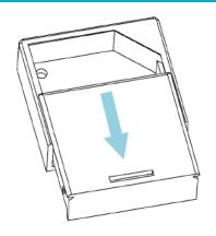
Slide open the Door/Window Sensor's housing. Install the CR2032 battery in the top part as shown below.
